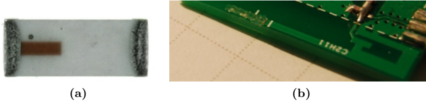
Figure 2.10: Commercial antennas for small devices at 2.4 GHz: (a) Ceramic Chip Antenna, from Johanson Technology (2450AT42A100) and (b) F inverted antenna, from Texas Instruments (DN0007)
