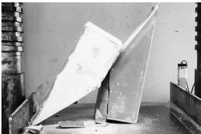
Fig. 6a) Adhesive failure
