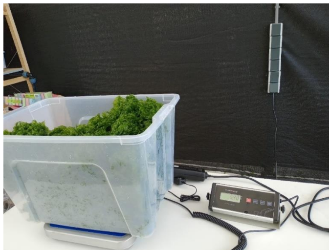
Figure 26 – Weekly biomass sampling from the tanks, used for subsequent analysis of growth rates (DGR%) and assessment of seaweed quality. Photo: Paulo Pereira
