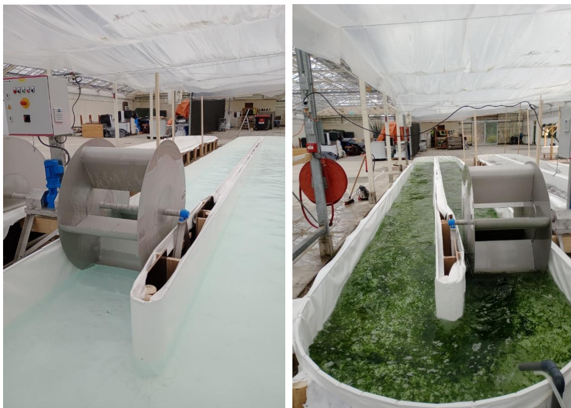
Figure 34 – On the left, a photo of the raceway after completion, filled with water for leak testing. On the right, the raceway after successful testing, with Ulva spp. introduced to initiate production. Photo: Paulo Pereira
