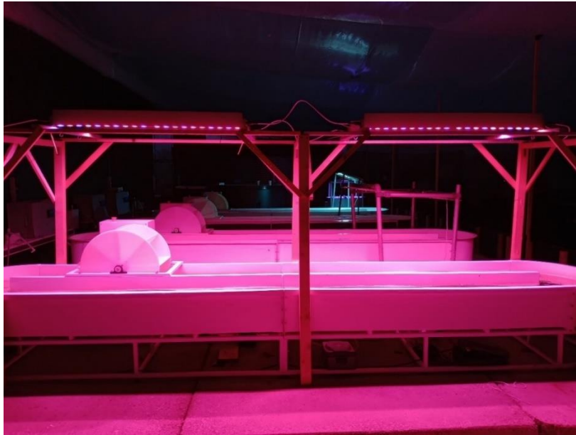
Figure 19 – Philips red/pink spectrum lighting system, utilized to investigate and enhance growth performance and physiological responses of macroalgae under specific wavelength conditions. Photo: Paulo Pereira
