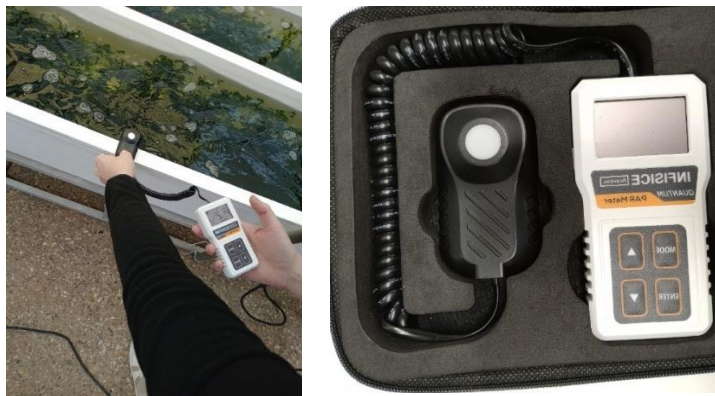
Figure 16 – Light monitoring in the Ulva raceway (left). Infisice Quantum PAR Meter (right). Photo: Paulo Pereira
