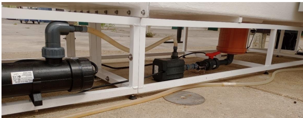
Figure 36 – Water recirculation system equipped with a 600 liters/hour recirculation pump and UV sterilization unit. Photo: Paulo Pereira.
