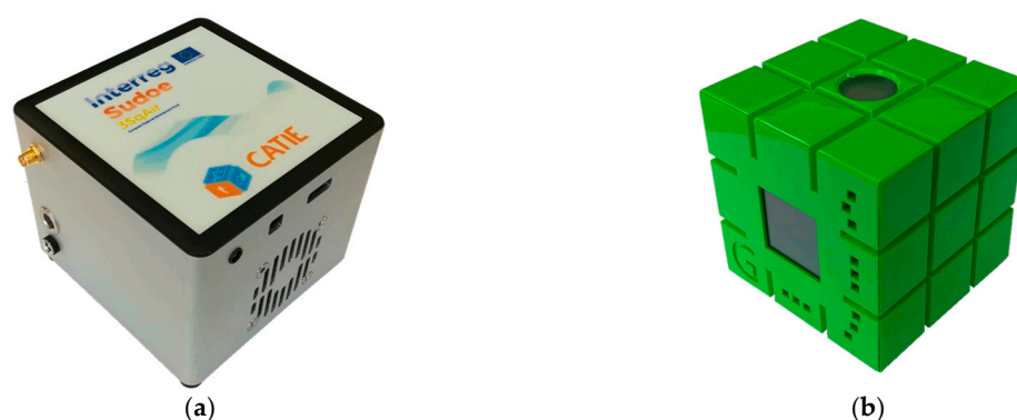
Figure 6. Monitoring device: (a) Image of a Catie IEQ box. (b) Image of a GreenMe cube.
