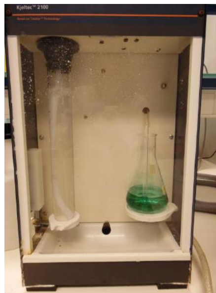
Figura 7.1.5 – Destilador (Foss, Kjeltec TM 2100, Tecator Technology).
