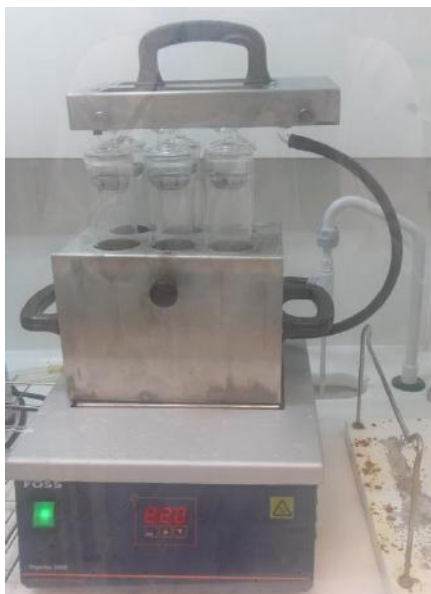
Figura 7.1.4 – Digestor (Digestor 2006 Foss, Tecator Technology).
