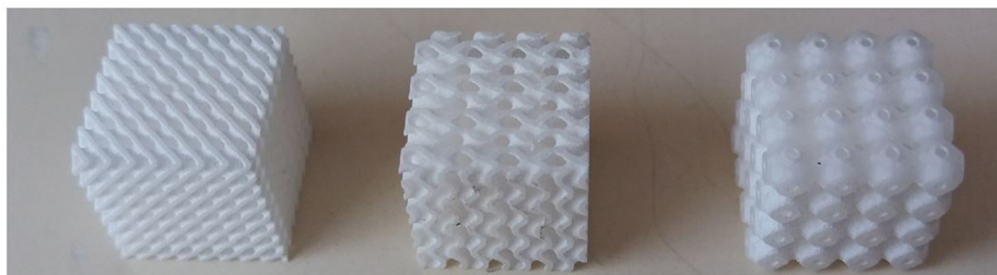
Fig. 1. Example of a 3D printed SD60, SG60 and SP60 scaffolds.
