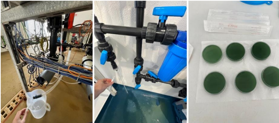
Figure 43. Microbiology sampling: post-UV running seawater of Technical area (left) and post-cartridge filter in Larvae room (middle); TCBS plates for the harvest tanks sampling of the Upright Bag room (right) (Source: Author, 2025).
