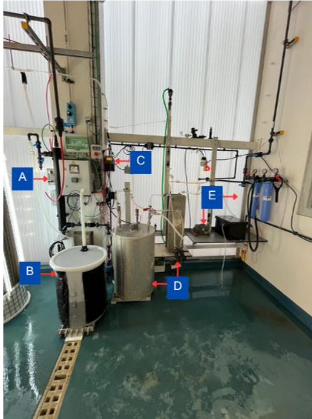
Figure 23. Supply system: CO 2 flowmeter (A), nutrients tank (B), nutrients dose pump (C), pasteurizer and heat exchanger (D), water pump and cartridge filters (E) (Source: Author, 2025).
