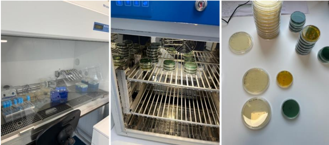
Figure 44. Sample processing in the laminar flow cabinet (left), storing in the controlled-temperature oven (middle), and reading (right) (Source: Author, 2025).
