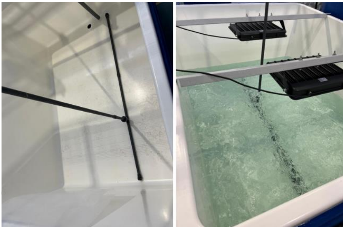
Figure 45. Batch tank configuration with PVC aeration pipe bars and LED lamps (Source: Author, 2024).
