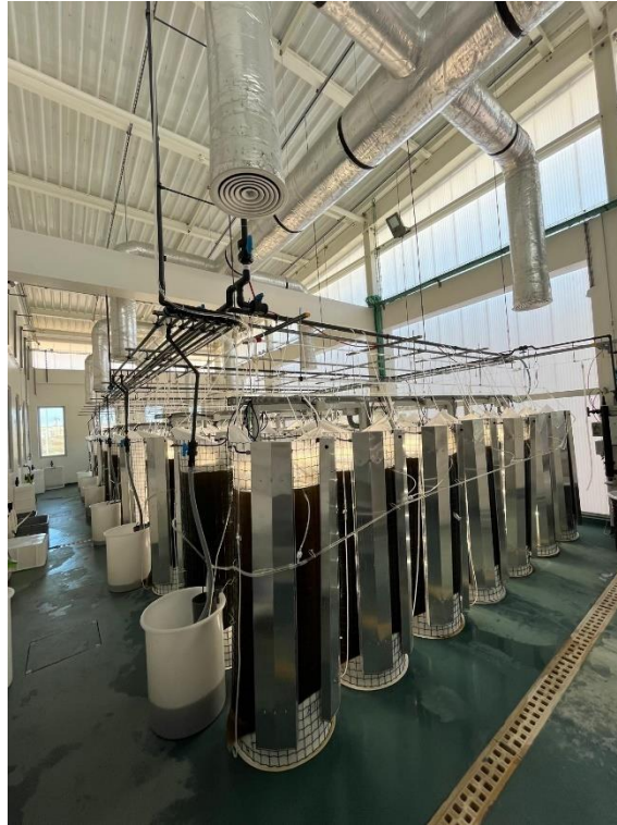
Figure 18. Upright Bag room, showcasing the six existing lines of bags and their respective harvest tank (Source: Author, 2025).
