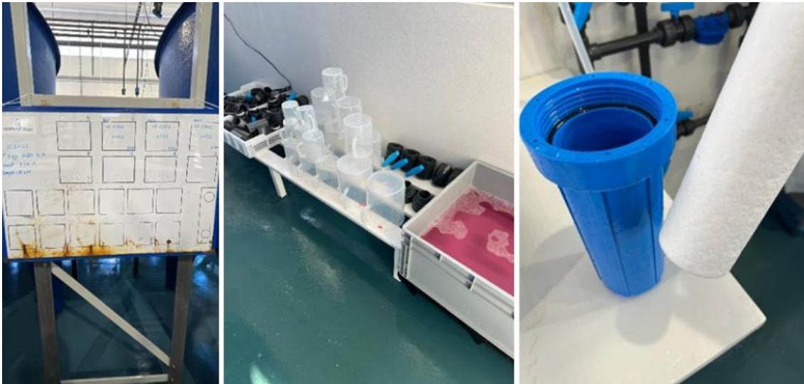
Figure 37. Data board (represented day 12) (left); cleaned and disinfected material (middle); and the weekly cartridge filter change (right) (Source: Author, 2025).
