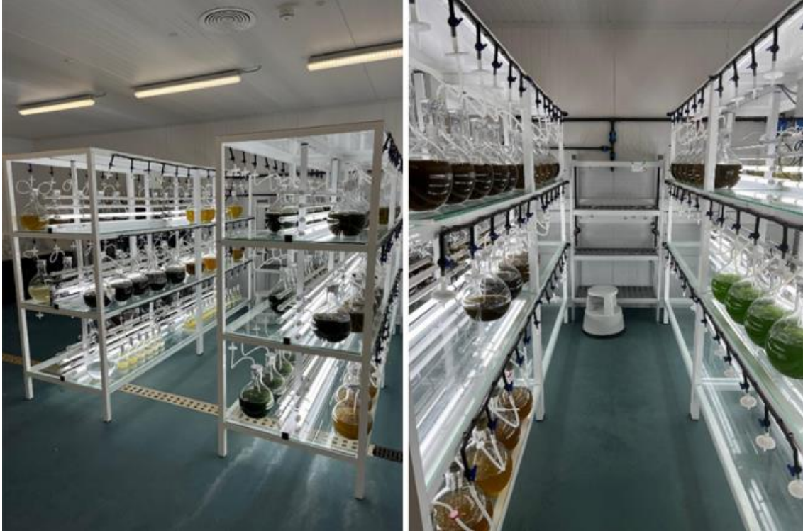
Figure 15. Balloon shelves supplied with aeration, CO 2 and light (Source: Author, 2025).
