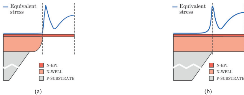
Fig. 1. Characteristic equivalent stress on the surface of a membrane with: (a) thickness given by the n -type epitaxial layer and area set by the diffused n -well layer; (b) thickness given by n -type layers and area defined by the bulk etch of the silicon wafer.
