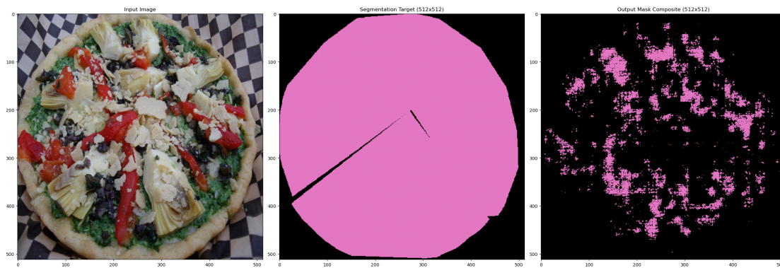
Figure 4.14: Example of segmentation results from the original ENet model. A pizza is represented. From left to right: original image, ground truth mask, mask from segmentation model.
