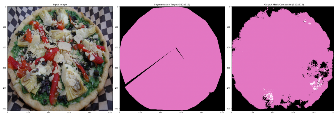
Figure 4.15: Example of segmentation results from the tuned ENet model. A pizza is represented. From left to right: original image, ground truth mask, mask from segmentation model.
