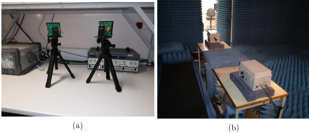
Figure 4.10: RF Front-end solutions: (a) VUBIQ PEM009 and (b) IT.
