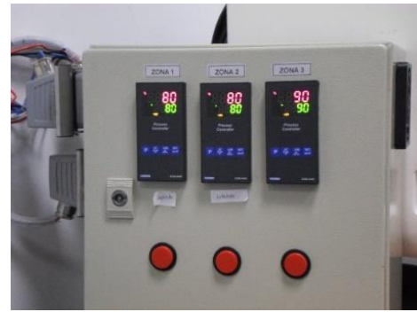
Fig. 7. Thermostat system, settled for the configuration “80-80-90”, after 8 minutes of footage.
