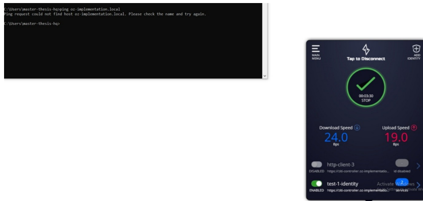
Figure 37: Unsuccessful attempt to access an unauthorised service (DC #1)
