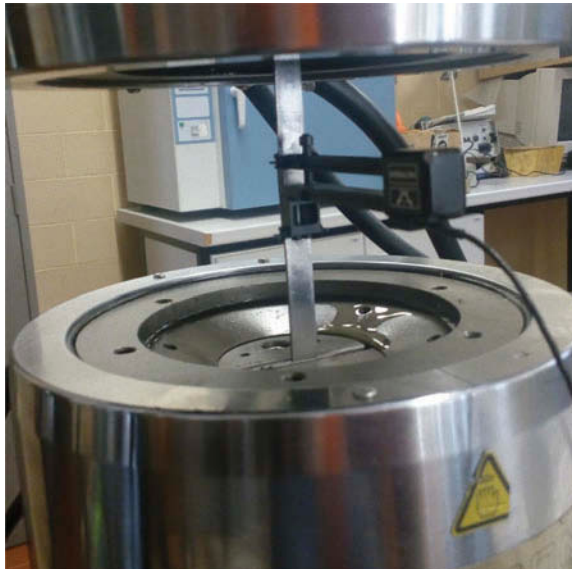
Figure 3. Experimental setting showing the specimen clamping grips and the extensometer coupled to the specimen.
