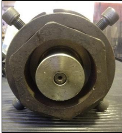
Figure 33 – Extruder head mounted
