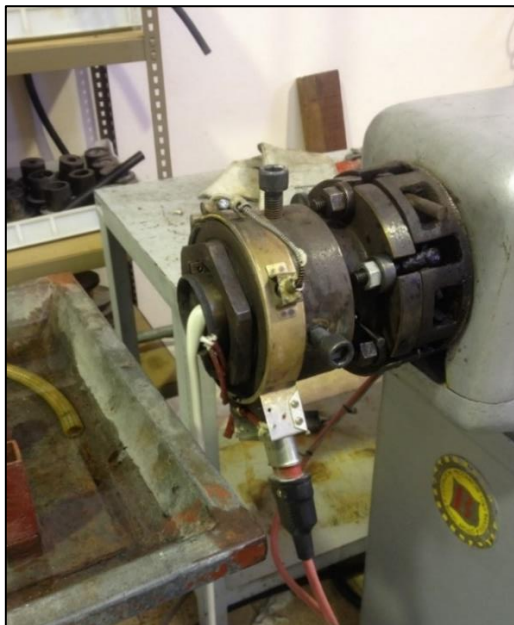
Figure 34 – Die head extruding PP
