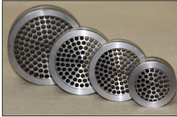
Figure 7 – Extruder breaker plate [8]
