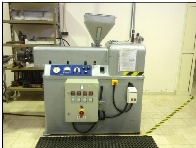
Figure 19 – Single Screw Extruder
