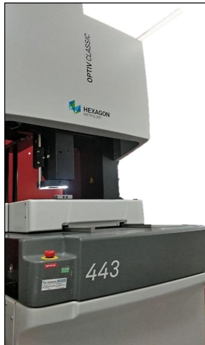
Figure 24 Optiv Classic 443 tp CMM used in the work
