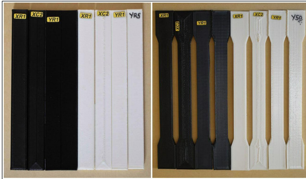
Figure 30 Bending specimens [Right] and Tensile specimens [Left] produced.
