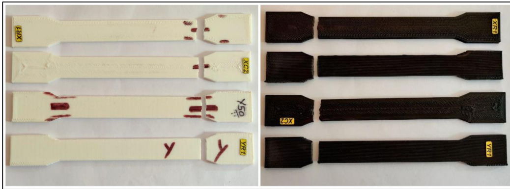
Figure 37 ABS [Left] and ASA [Right] Samples after the Tensile test.
