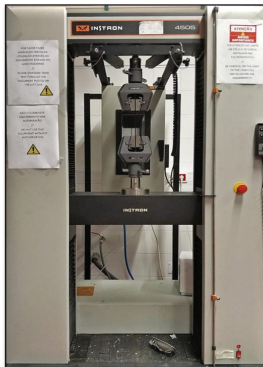
Figure 36 Instron 4505 universal testing machine used for conducting Tensile, Bending and Compression tests for the work
