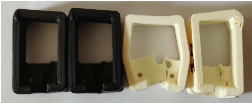
Figure 54 ASA [Left] and ABS [Right] parts after the Compression test.
