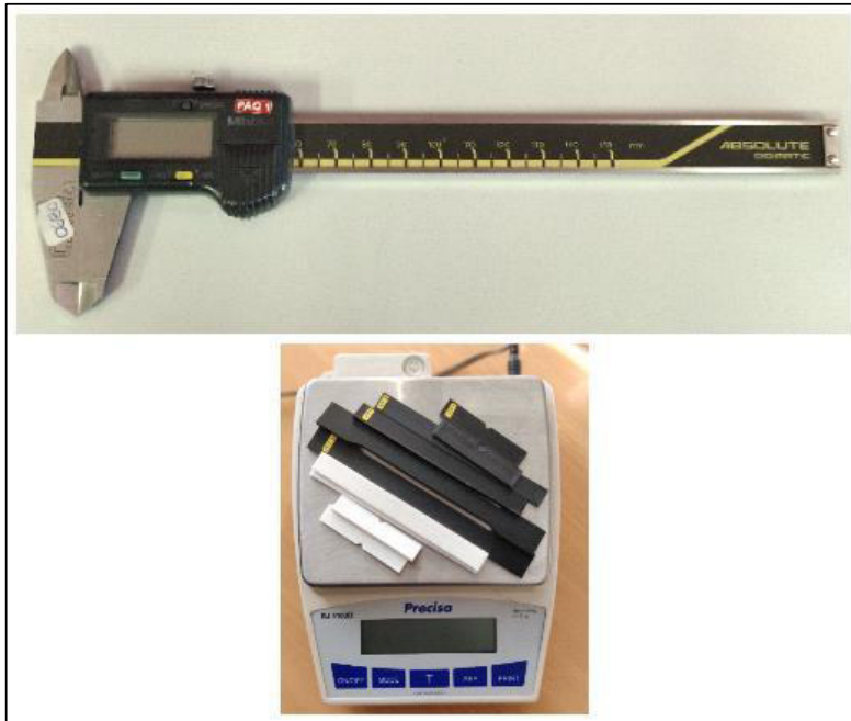
Figure 27 Digital caliper (top) and weighing scale (bottom) used for the measurement of the specimens
