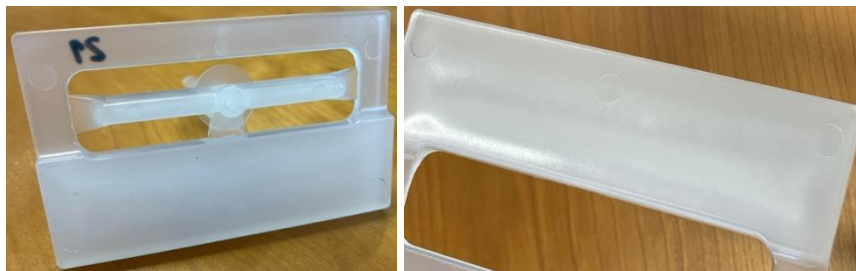
Figure 4-15 – Parts injected in PP and resulting shrinkage and warpage.
