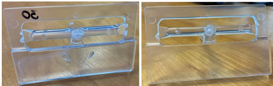
Figure 4-11 – Parts injected in PS and effects of changing injection speed. Voids (left) and their mitigation (right).
