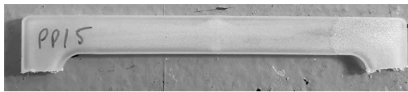
Figure 3-12 – Example of specimen geometry used in Charpy and tensile tests.
