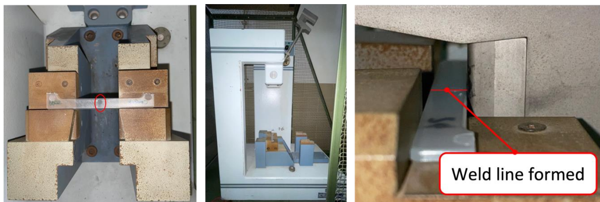
Figure 4-23 – Charpy test specimen setup onto the CEAST impact tester.
