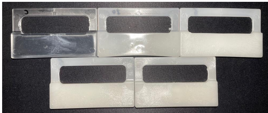
Figure 4-13 – Top view of PS parts with and without blowing agent. PS, PS-BA0.5, PS-BA0.8, PS-BA1.0, and PS-BA1.5 (shown left to right and top to bottom).
