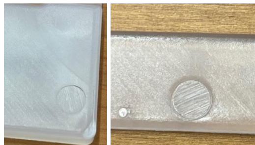
Figure 4-16 – Welding lines zones of parts injected in PP.
