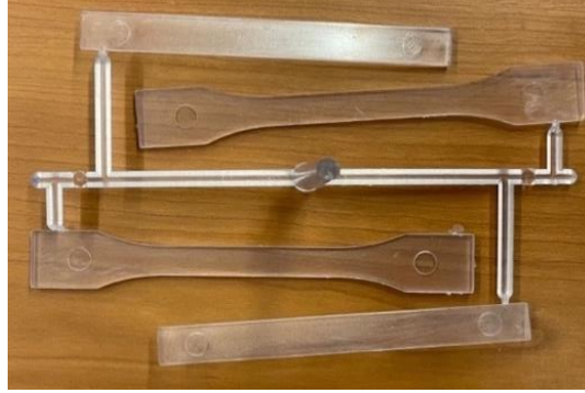
Figure 3-22 – Example of the geometry of the injected geometry.
