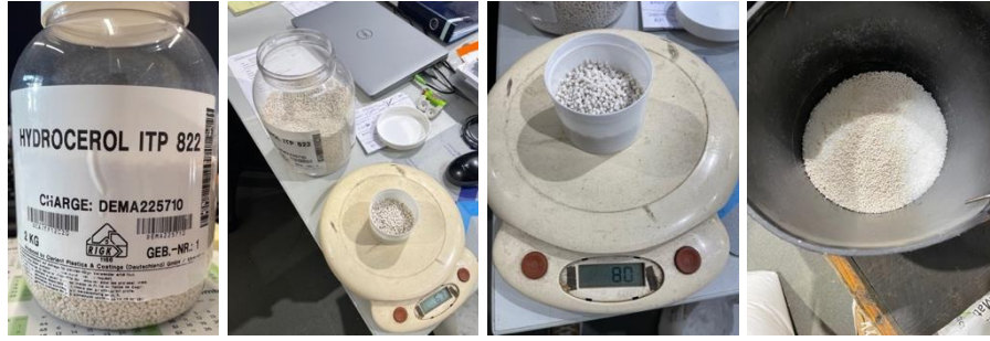
Figure 4-17 – Mixing process of the blowing agent.
