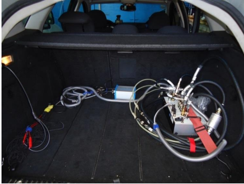
Figure 4 - Details of the fuel metering equipment (Kistler Datron DFL3x - 5bar) installation in the trunk of the vehicle
