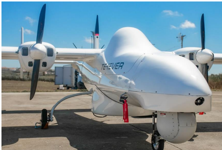
Figure 12 - Tekever AR5 with a solid spring landing gear [21].
