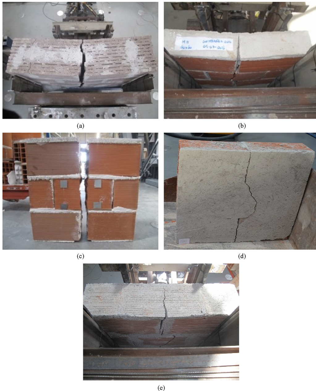
Fig. 23 Flexural strength tests parallel to horizontal bed joints failure modes: (a) VHC315; (b) HCHB110; (c) HCHB150; (d) HCHB150P10 (existing); (e) HCHB150 (existing).
