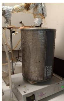
Figure 2.5. Vertical furnace (Thermolyne, model 21100).
