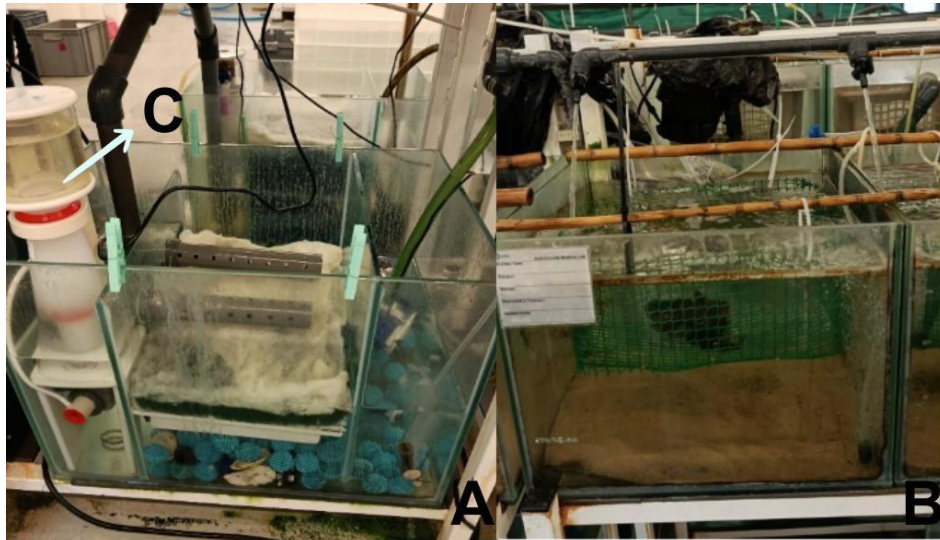
Figure 2.7- A- SUMP tank setup used in this trial (C-Skimmer); B- Plastic basket with mussels.
