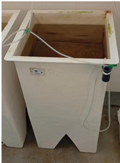
Figure 2.1- 50 L flat-bottom fiberglass tanks used for Hediste diversicolor reproduction and growth of larva and juveniles.
