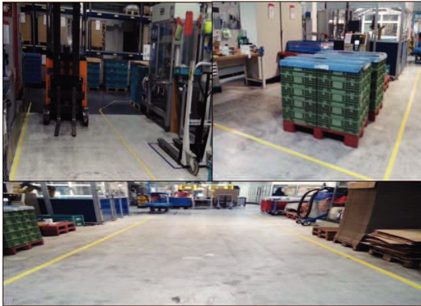
Figure 39 - Yellow marks on the floor for the transport way.
