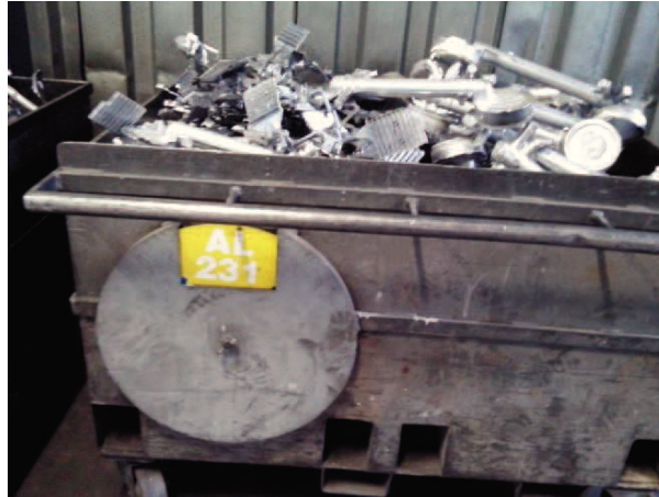
Figure 21 – Container with the recycled material, identified with number and color of aluminium alloy.
