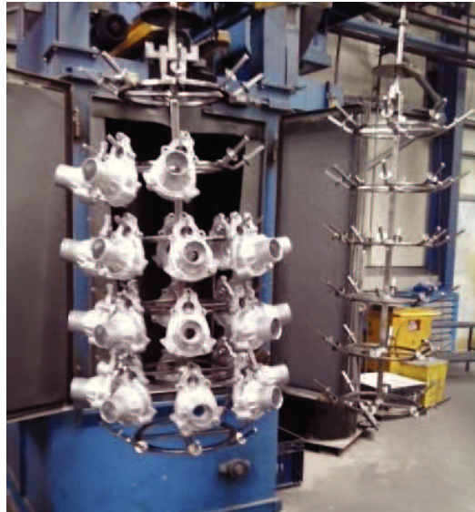
Figure 26 – Shot peening machine with the two supports outside.
