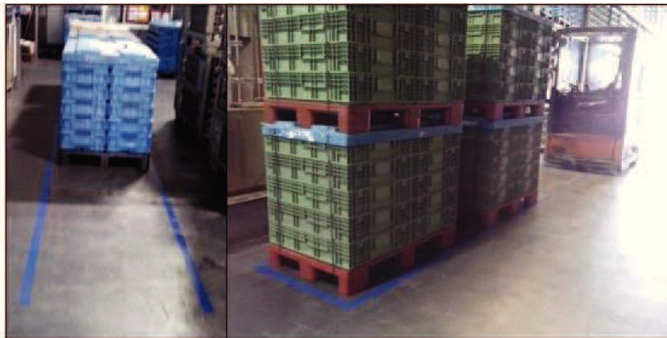
Figure 40 - Blue marks on the floor to bound pallets area before packing (left) and after (right).
