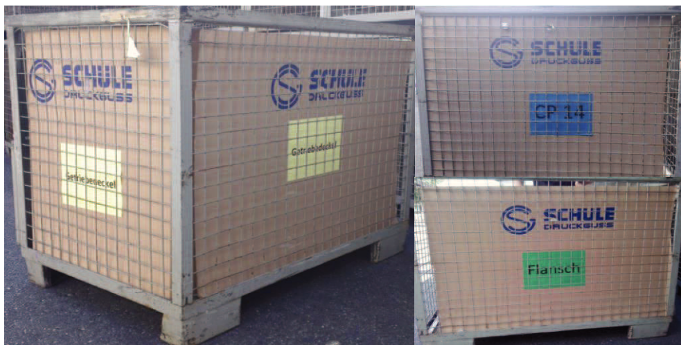
Figure 56 – Color system to mark the grid boxes with the raw parts.
