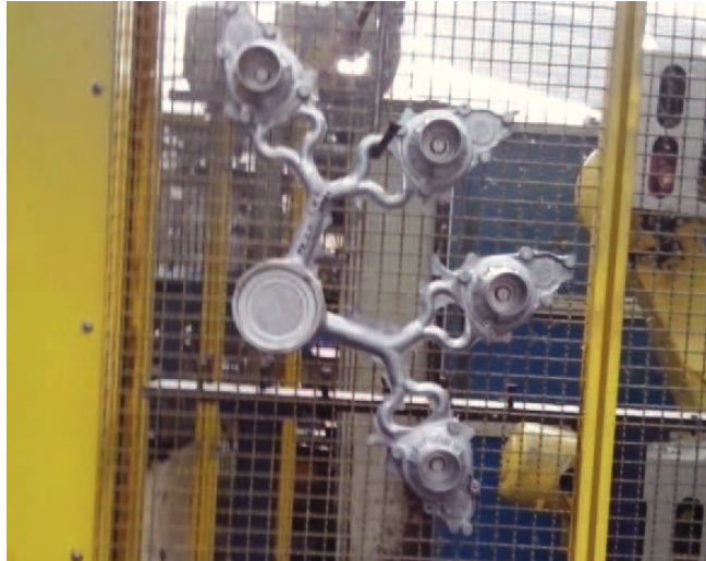
Figure 24 – Product structure after the die-casting process.
