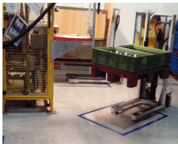
Figure 42 – Marking system for the Small Load Carrier on GM Delta production line.
