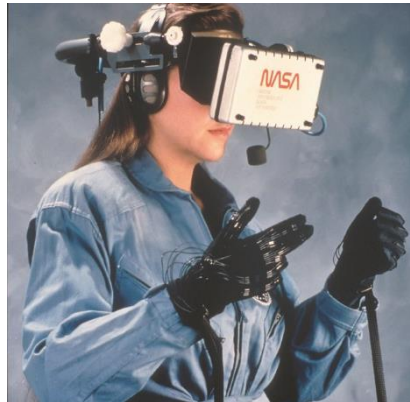
Figura 30 - Sistema VIEW (Virtual Interface Environment Workstation). Fonte: The Virtual Interface Environment Workstation (VIEW), 1990 | NASA
