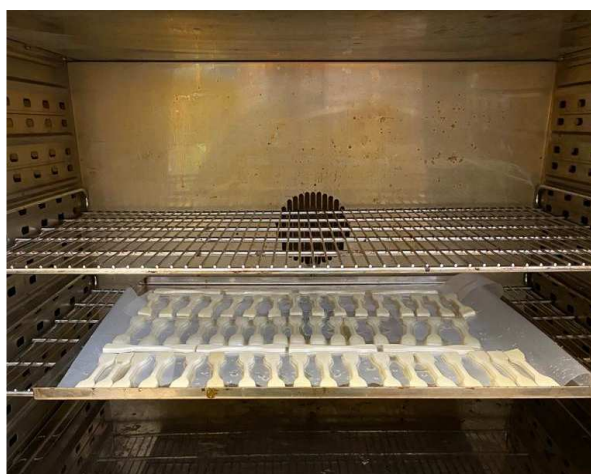
Figura 58 – Provetes na estufa HEK-GMBH MCP-Vacuum
