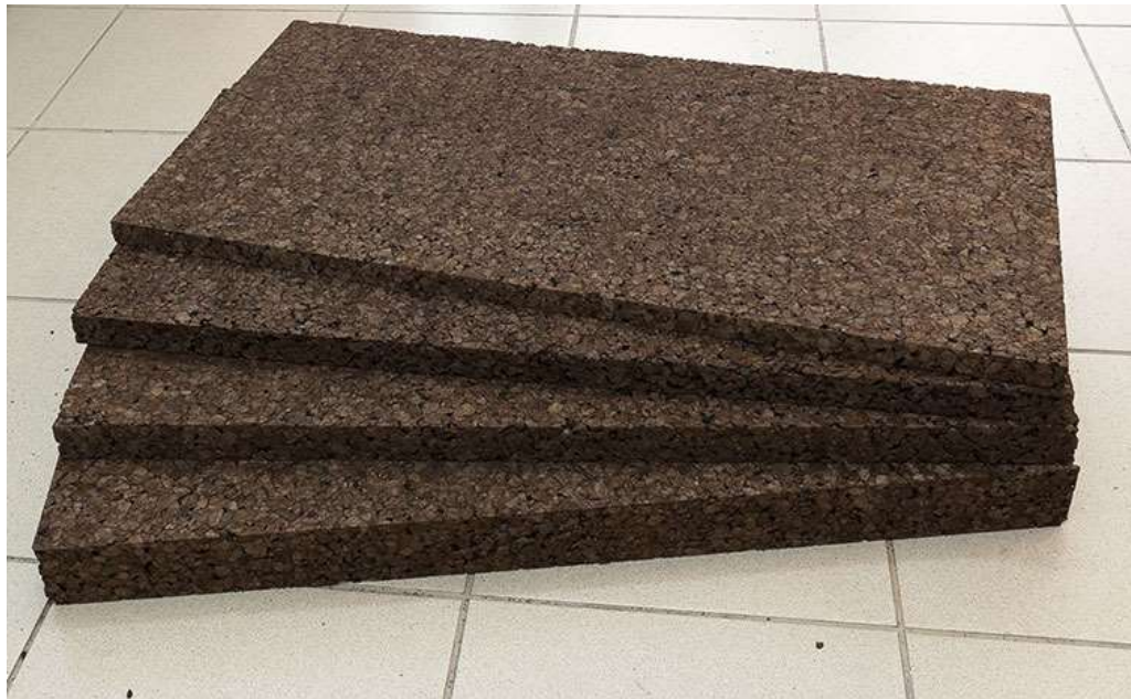
Figure 2.11. - General view of the cork plates
