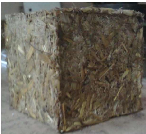
Figure 4.6. - General view of a sample-cube based on moss and straw
