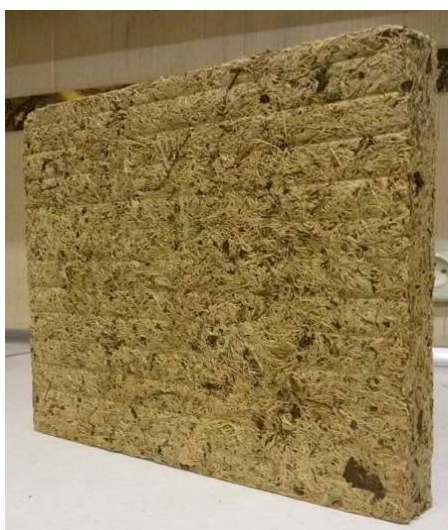
Figure 4.1. - Thermal insulation plates based on moss
