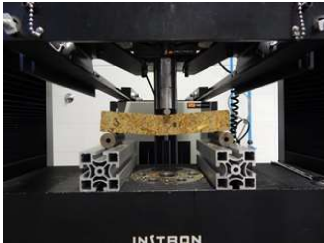
Figure 4.10. - General view of testing of beam samples for bending strength
