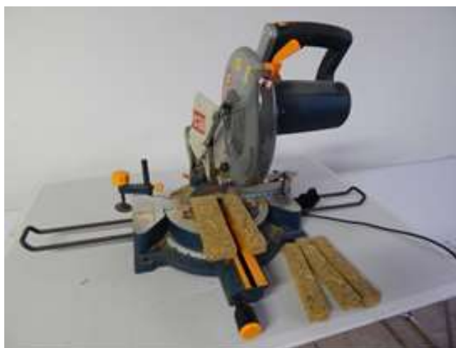
Figure 4.9. - Manufacturing of beam samples for bending strength test
