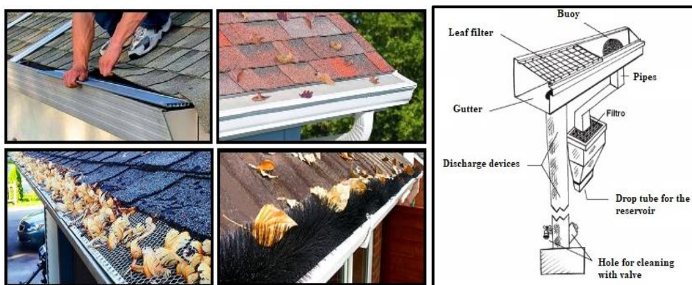
Figure 3.5 - Components of rainwater harvesting system
