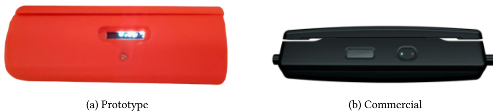
Figure 5: Versions of the GripWise dynamometer. Adapted from (Fernandes, 2022)
