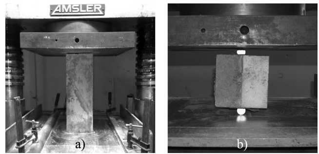
Fig. 3—Concrete specimens: (a) slant shear; and (b) splitting.
