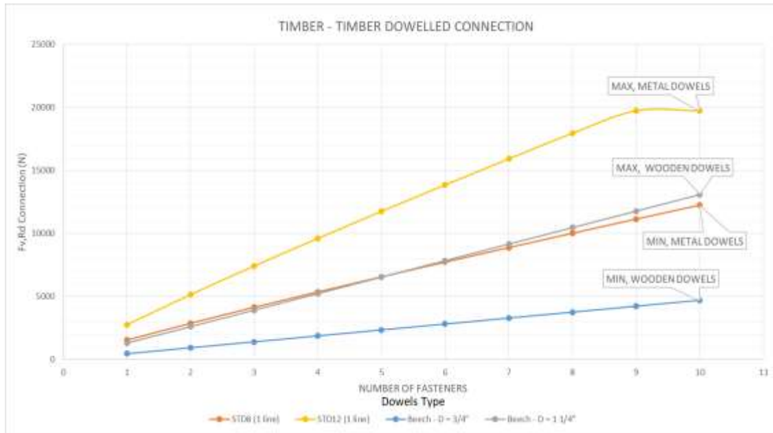
Figure 5.22 Influence of Type of Fastener in a Timber – Timber Dowelled Connection (Mortise and Tenon Connection)
