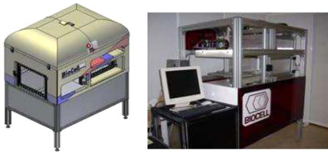
Fig. 1. BioCell Printing device: (a) CAD model; (b) functional prototype.
