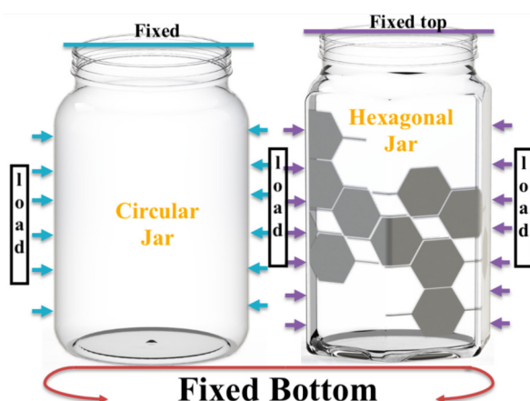
Figure 5.3: Boundary condition - Squeeze test
