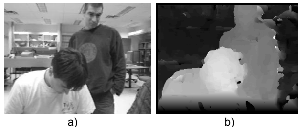
Fig. 3. Bumblebee2 stereo system, a) is the source of chromatic images and b) their depth map [3]
