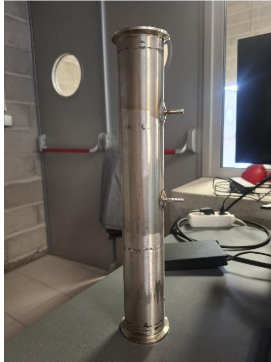
Figure 47 - Venturi Tube in Inox
