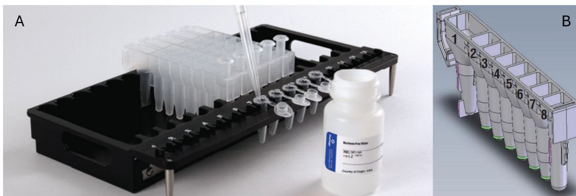
Figure 4 – A) Setup and configuration of deck tray; B) Maxwell® RSC Cartridge (Source: Promega Corporation (2022)).
