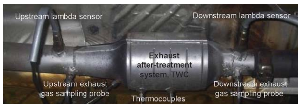
Figure 2. Photograph of the exhaust after treatment system showing the TWC, the exhaust gas sampling probes, the lambda sensors and the thermocouples.
