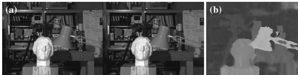
Fig. 5 a Two different views of the same scene and b corresponding disparity map
