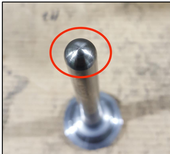
FIGURE 26: Plunger defect on top radius (depth of cut 0.1 mm)
