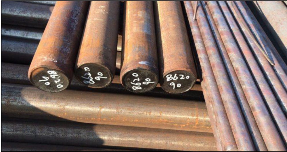
FIGURE 15: Raw material (AISI 8620 Steel) to be metallised and machined
