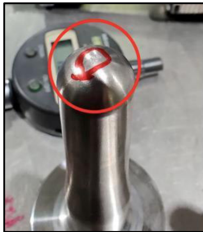
FIGURE 25: Plunger defect on top radius (depth of cut 0.09 mm)
