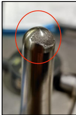
FIGURE 27: Plunger defect on top radius (depth of cut 0.15 mm)
