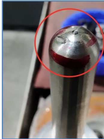
FIGURE 24: Plunger defect on top radius (depth of cut 0.07 mm)
