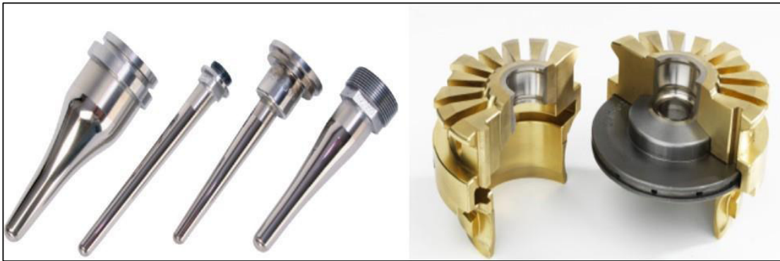
FIGURE 12: Plungers for blank moulds (Left) and Neck and Guide rings for Plunger Insert (Right) The Plunger is responsible for managing the flow of glass inside the container and the Guide Ring is the part which makes the top of bottle whereas the Neck Ring is a threaded component [34][35]
