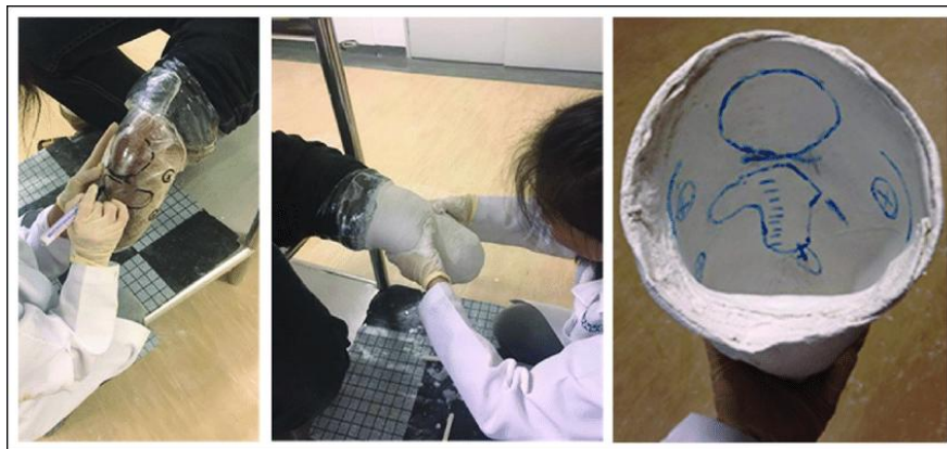
Figure 9. Traditional method of plaster impression (Source: Mehmood, Abd Razak, Gholizadeh, & Chung, 2018, Figure 2).
