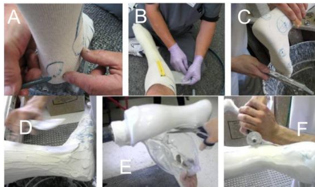
Figure 14 . Conventional method for fabricating ankle-foot orthosis for a patient (Source: Mavroidis, et al., 2024, Figure 1).
