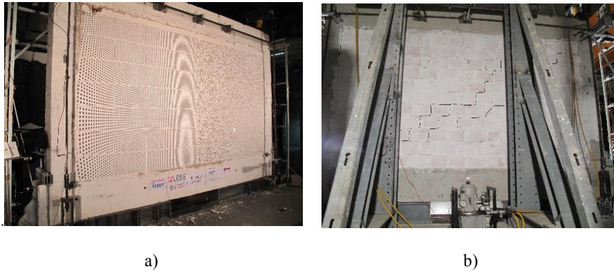
Fig. 8: In-plane final cracking pattern: a) Stronger panel ( t=150\text{mm} ) and b) weaker panel ( t=110\text{mm} ).
