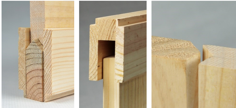
Fig. 1. Early prototypes of the 1C system: lower and upper sockets in the “U” shape rail, made of pine wood; fittings between vertical boards, whose “V” shaped profile guarantees a perfect fit (photos: Pedro Cá).
