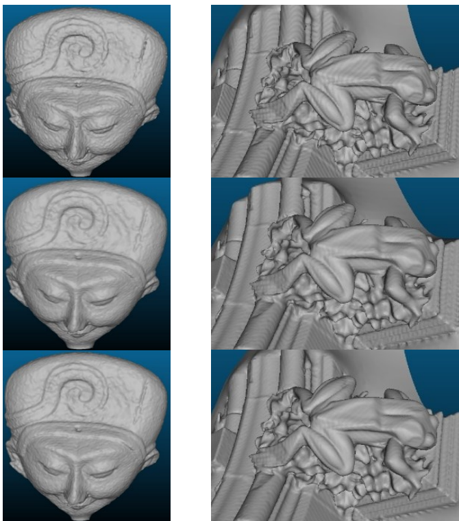
Fig. 6. Comparison of the reconstructed surfaces using the reference method with \alpha=4 (top), using only the GT regularization term \lambda=0.01 (middle) and the proposed solution combining the two regularization terms with \alpha=4 and \lambda=0.01 (bottom), for Egyptian mask and Frog67 point cloud datasets.
