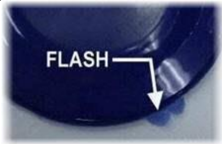
Figure 29- a part with flashes in it.[17]
