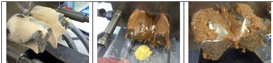
Fig. 9 – Appearance of the materials inside the plastograph mixer along the process of optimization of composites:
