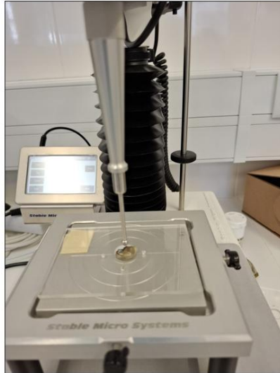
Figure 10 - Texture profile analysis (TPA) of an oyster muscle sample, using a texturometer.
