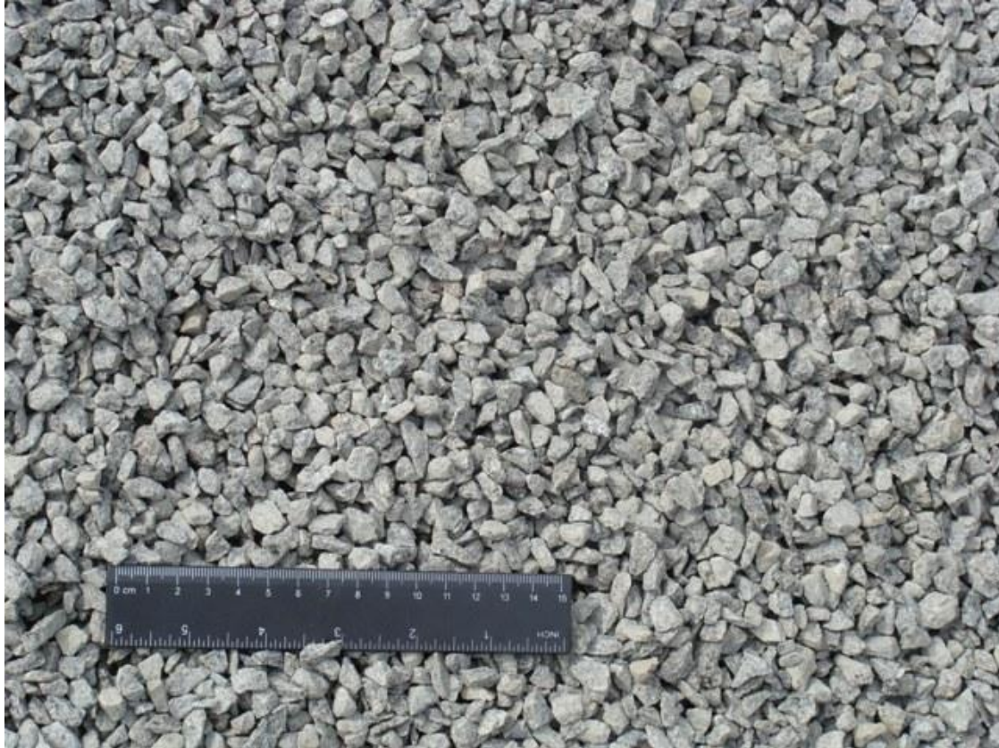
Figure 21. Fractional screening of crushed stone
