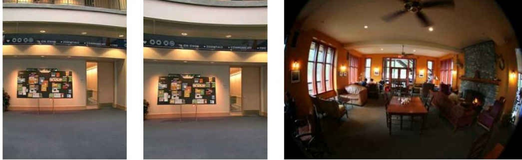
Figure 4: Radial lens distortion. From left to right, barrel, pincushion and fisheye distortion, Szeliski, 2021
