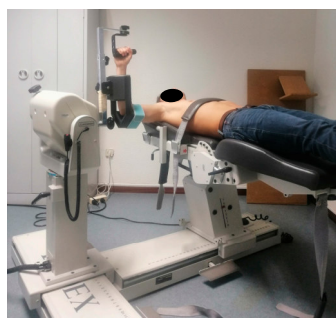
Figure 3. Subject position and stabilizing during the isokinetic dynamometer strength assessment.
