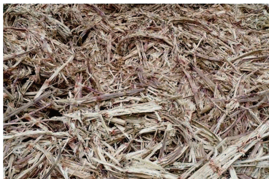
Figure 3: Pile of bagasse waste
