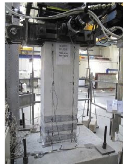
Fig. 1. a) RC column specimen dimensions and reinforcement detailing; b) General view of the test specimen at LESE laboratory.
