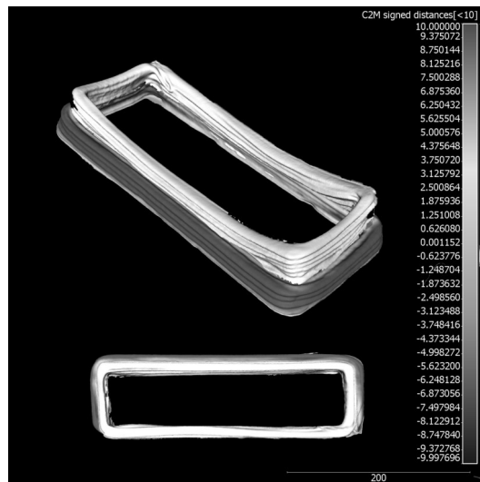
Figure 4.15: Deviation Analysis of Glass Fiber Composite
